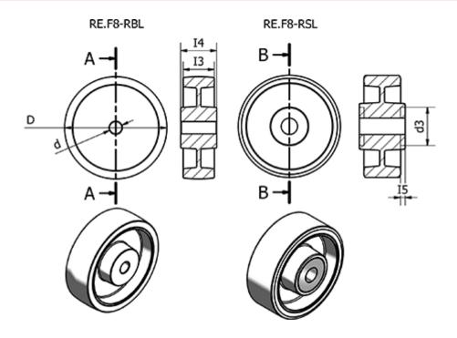
Code = 449453 d = 200 d3 = 47 Dynamic carrying capacity (N) = 9000 l3 = 50 l4 = 56 l5 = 13 Rolling resistance (N) = 6500Static load = 10000
